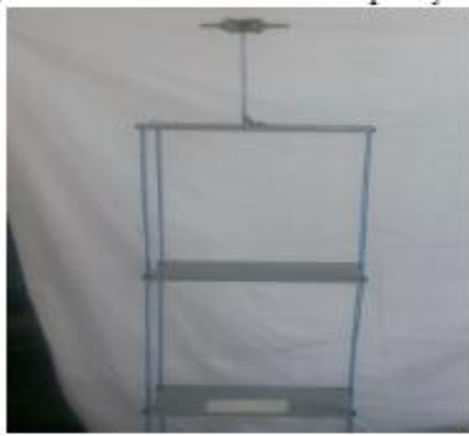
Fig -3: Structure with tuned mass damper
