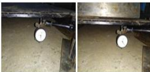
Fig 16: Dial gauge set to "0" before loading the Std. Steel pallet
