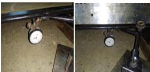
Fig 18: Dial gauge set to "0" before loading the
