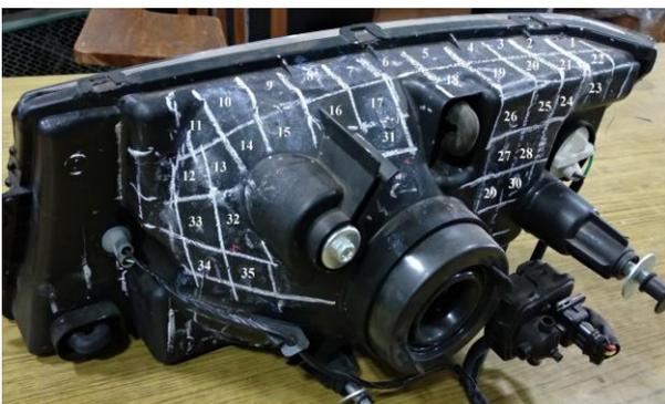
Fig-3: Grid formation on the back cover of headlamp
