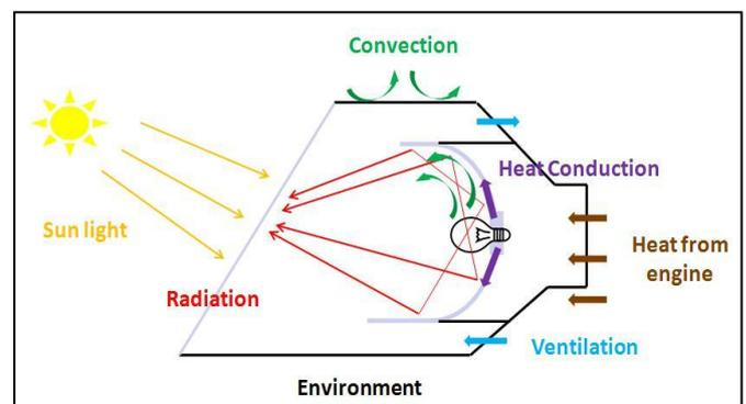
Fig-2: Mechanism inside the headlamp
