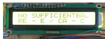
Fig -13: If entered amount is more than the available amount, then controller tells user to recharge
