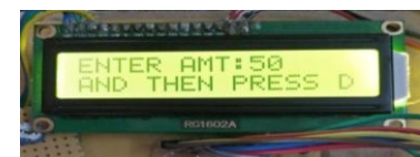
Fig -11: Controller asking the user to enter the amount of the petrol
