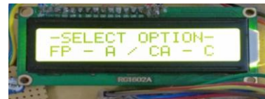
Fig -10: Controller asking the user to press the key to fill the petrol or to cancel the action
