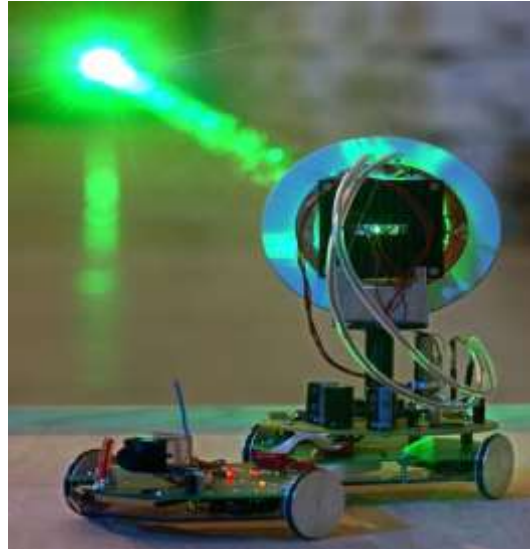
Figure 5: EADS developed, fully laser powered autonomous rover. (Source: EADS) [10][11]
