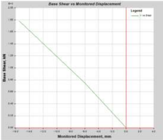
Figure 7 Base shear v/s Displacements in Push X After Analysis in for Irregular Building with Shear Wall
