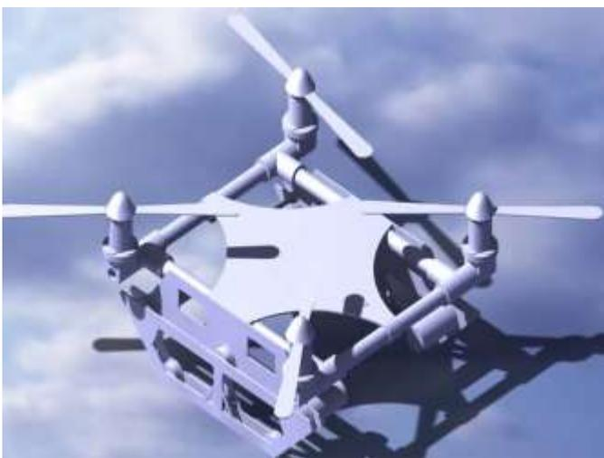
Fig No. - 10: rendered view of tank-copter
