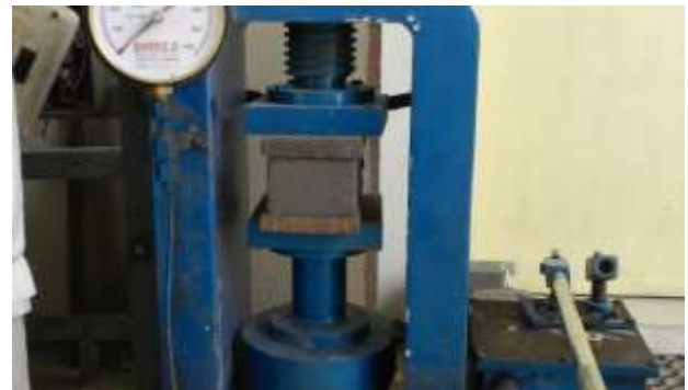
Figure: Placing of concrete cube specimen in Compression testing machine.
