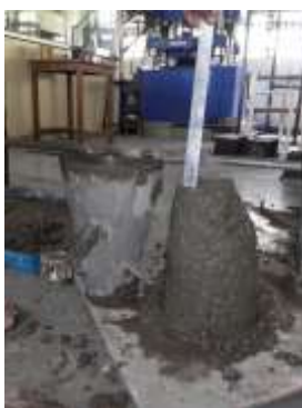
Fig 3: Workability test of concrete by slump cone method
