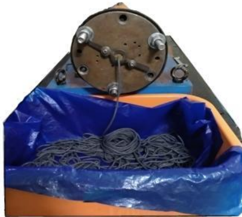
Fig -4: Silicon polymer with abrasive is extruded through specimen
