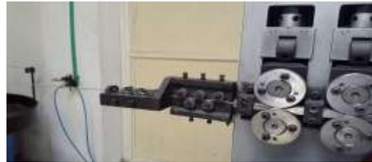
**Fig -10:** Wire Coiling Machine
