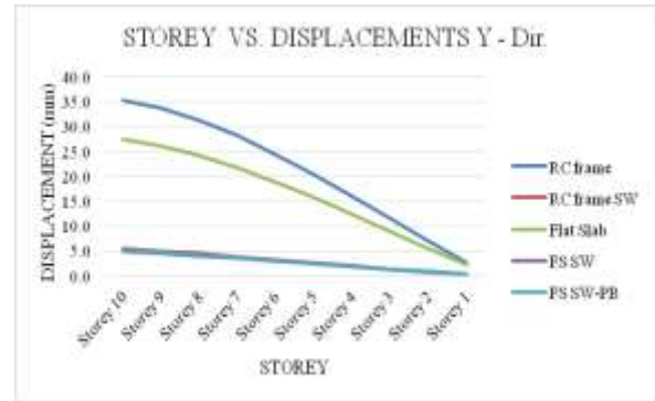
Fig -3: Storey vs. Displacement in Y-Direction
