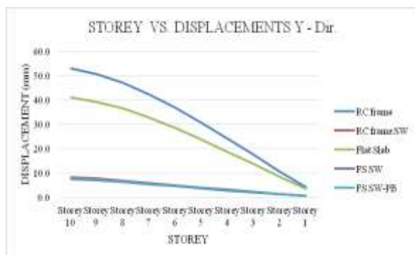
Fig -8: Storey vs. Displacements in Y-Direction
