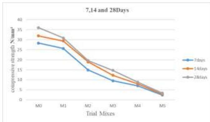
Fig 4.4 Compressive Strength Results for 7,14 and 28days
