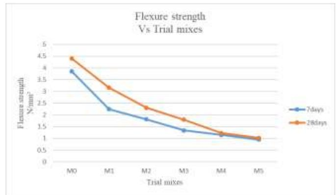
Fig 4.6 Flexure Strength Results for 7 and 28days of curing
