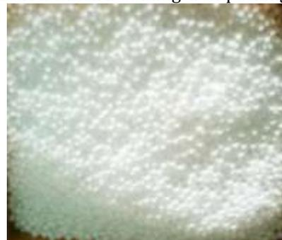
Fig 3.1 Expanded polystyrene (EPS)Beads
