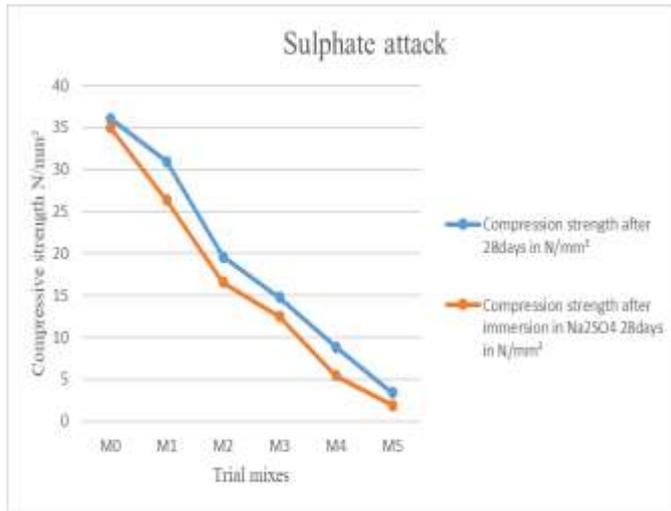
Fig 4.8 Sulphate Attack
