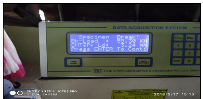
Fig. 5.7: Data acquisition on UTM for beam
