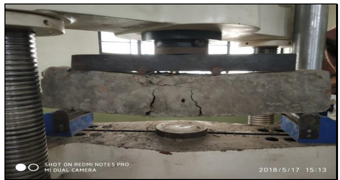
Fig. 5.6: Flexural Strength Test on Beam using Universal Testing Machine (UTM)
