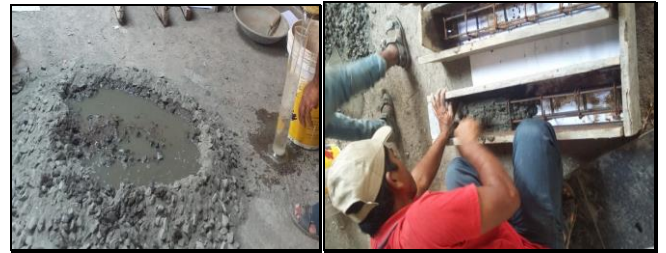
Fig.5.5: Preparation of Mix and Casting of beam specimens
