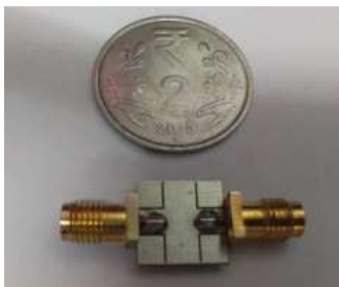
Fig. 6. Fabricated model of the proposed filter
