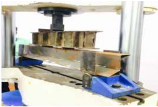
Fig 11 – Laboratory testing on THFB-1 Z – section
