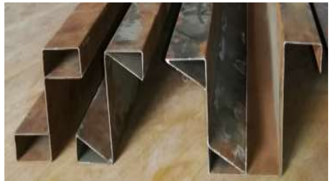
Fig 5 - Fabricated Test specimens
