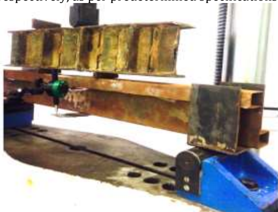
Fig 17 – Laboratory testing on RHFB Z – section
