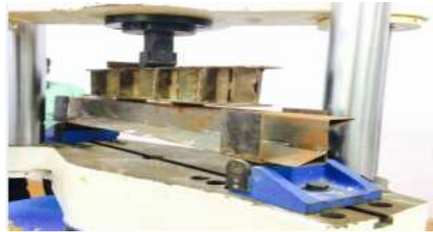
Fig 14 – Laboratory testing on THFB-2 Z – section
