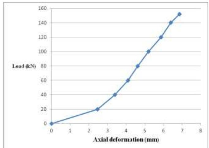
Fig-11: Load Vs Axial deformation graph of TFC- 0
