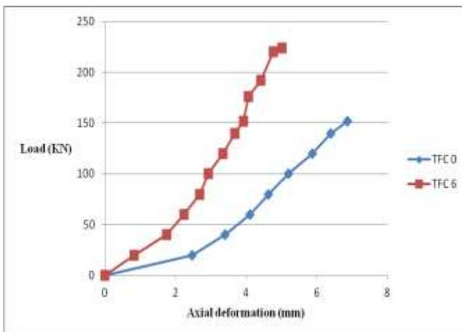
**Fig-14:** Load Vs Axial deformation graph of TFC-6
