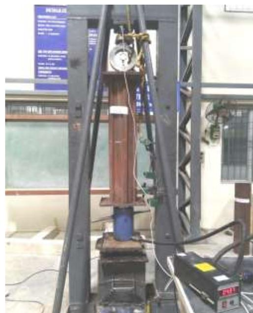
**Fig -6:** Experimental setup for TFC(s)
