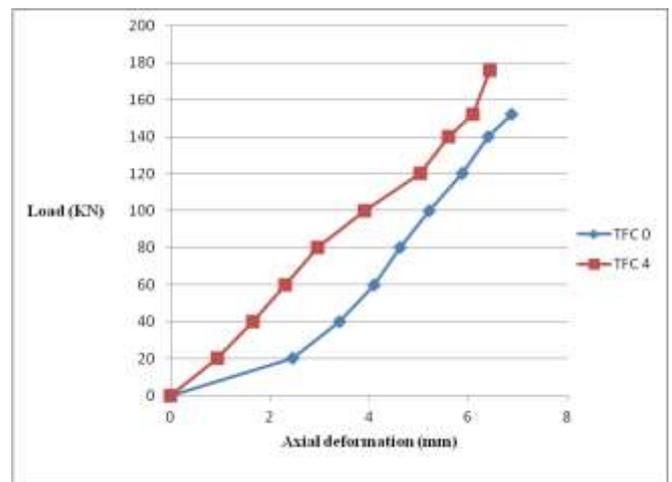
Fig-12: Load Vs Axial deformation graph of TFC-4
