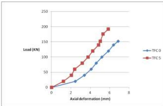
**Fig.13** Load Vs Axial deformation graph of TFC-5
