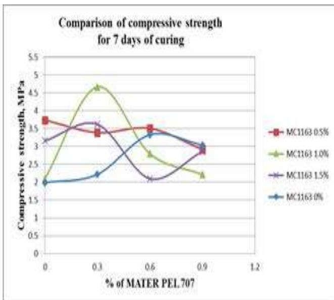
**Graph -1:** Compressive strength for 7 days cured compressed stabilized earth blocks in different chemical proportions
