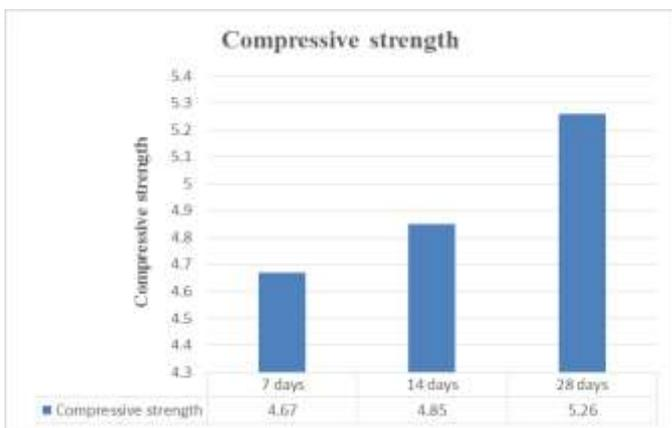
The result shows that the highest compressive strength of 5.260 N/mm<sup>2</sup> was obtained from sample at the curing age of 28 days.
