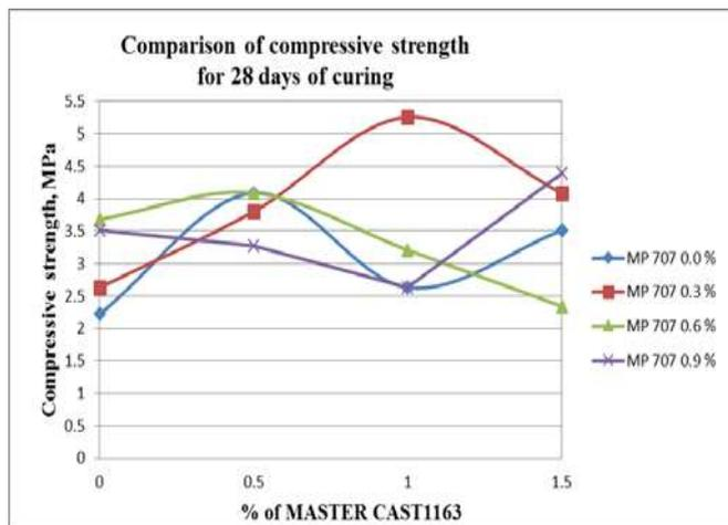
Graph -6: Compressive strength for 28 days cured compressed stabilized earth blocks in different chemical proportions.
