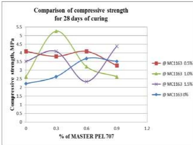
Graph -5: Compressive strength for 28 days cured compressed stabilized earth blocks in different chemical proportions
