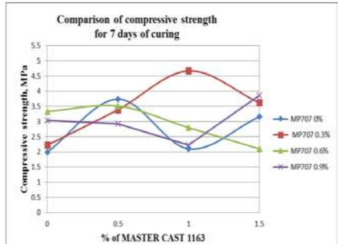
**Graph -2:** Compressive strength for 7 days cured compressed stabilized earth blocks in different chemical proportions
