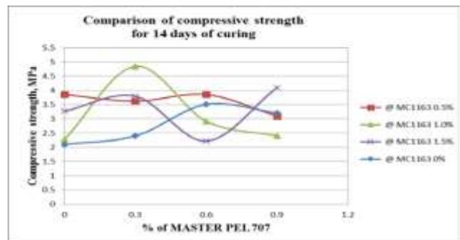
**Graph -3:** Compressive strength for 14 days cured compressed stabilized earth blocks in different chemical proportions
