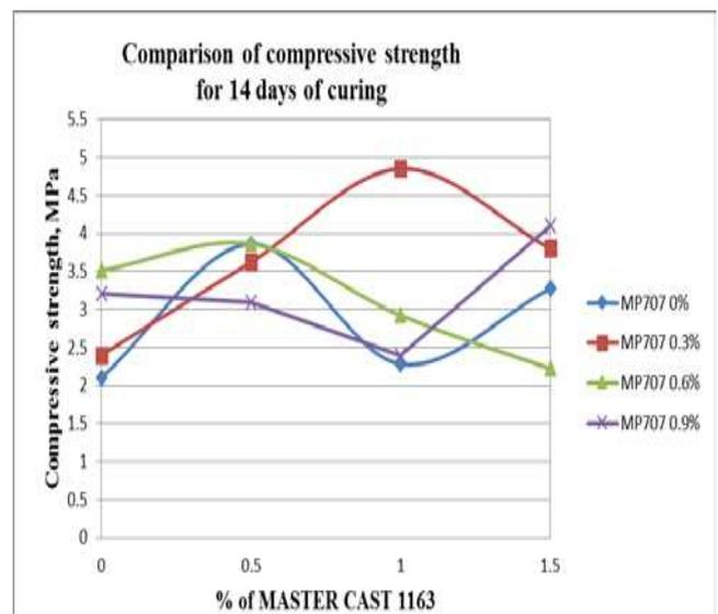
**Graph -4:** Compressive strength for 14 days cured compressed stabilized earth blocks in different chemical proportions
