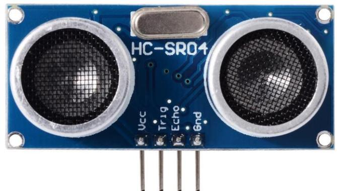
Fig -2: Ultrasonic Sensor (HC-SR04)
