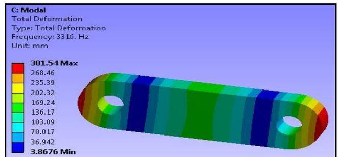
Fig.17 Natural frequency for the GFRP is 3316 Hz
