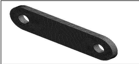
Fig.7 Meshed model chain link
