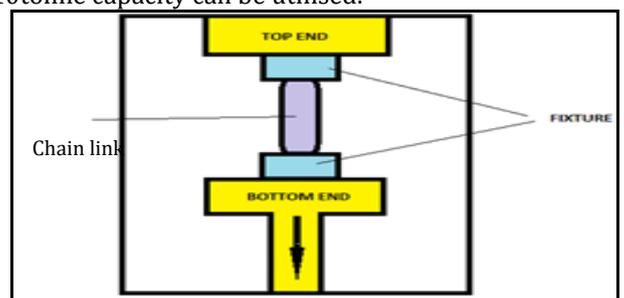
Fig.18 Testing GFRP Chain link on Universal Testing Machine
