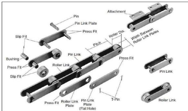
Fig. 1 Typical Roller chain Link Terminology
