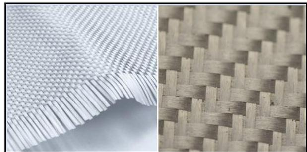
Fig. 3 Glass fiber in two different building formations
