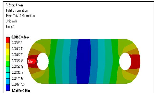
Fig.10 Total deformation plot for Steel chain link
