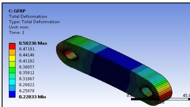
Fig.15 Total Deformation plot at GFRP chain link
