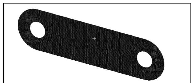
Fig.12 meshing glass fiber leaf spring shell 181
