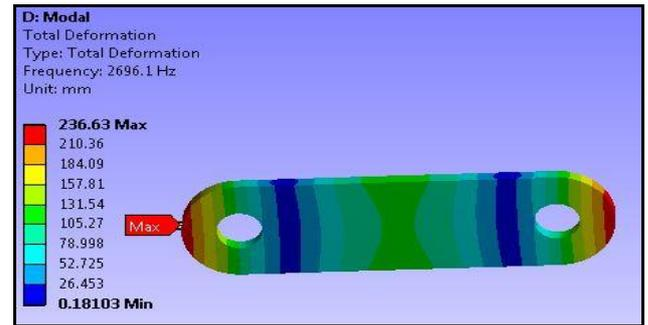
Fig.16 Natural frequency for the steel chain is 2696 Hz
