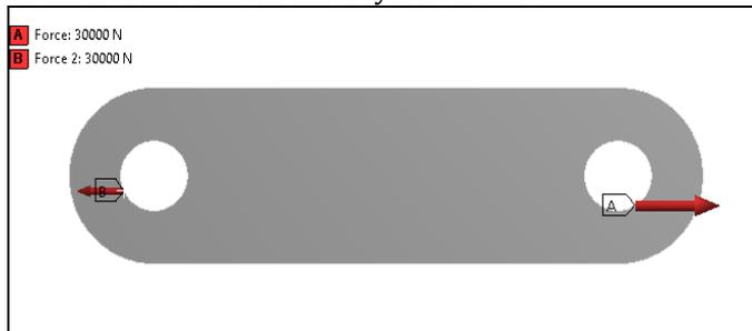
Fig.8 Boundary Condition and loading
