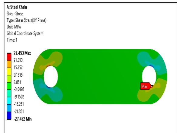
Fig.11 shear stress plot for chain link steel
