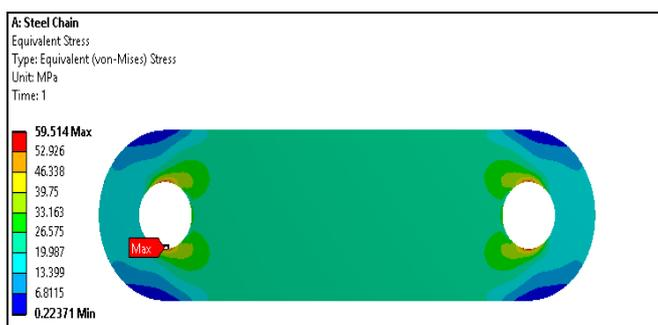
Fig.9 Von Mises Stress plot for Steel chain link
