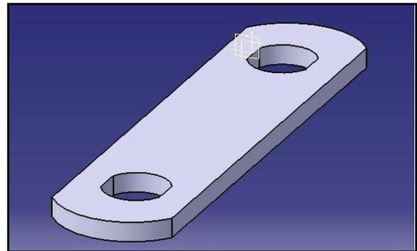
Fig. 4 Straight type chain link plate
