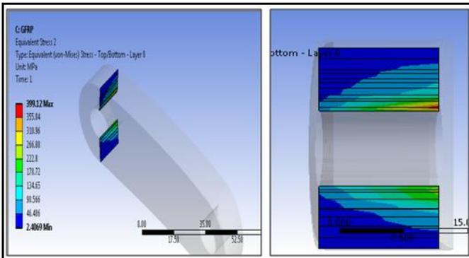
Fig.14 Average stress at the cross section
