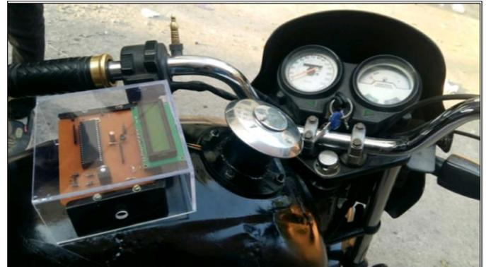
Fig -4. Digital Fuel Metering Device
