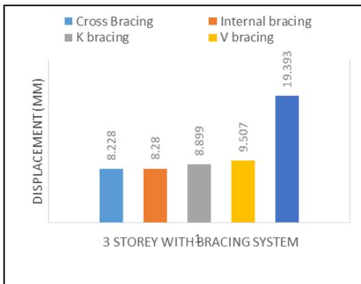
**Fig -6** Comparison of displacement for 3 storey model with bracing system.
