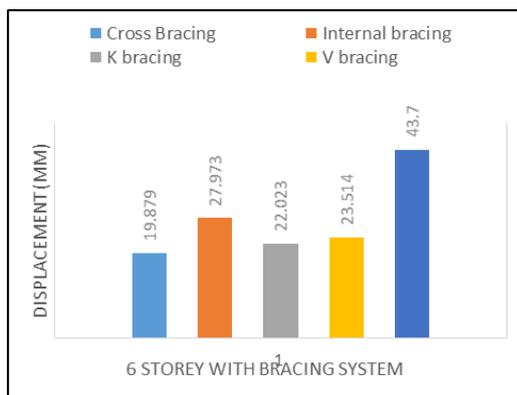
**Fig -7** Comparison of displacement for 6 storey model with bracing system.
