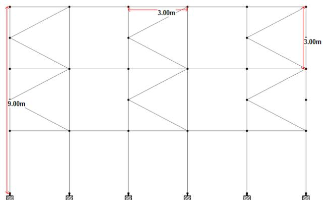
**Fig -4** Elevation of 3 storey with K bracing.
