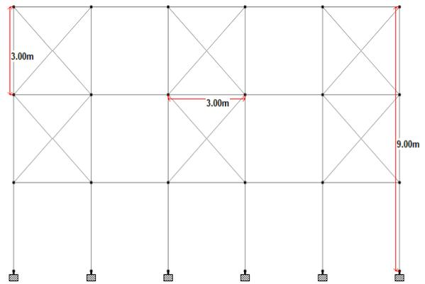
**Fig -2** Elevation of 3 storey with X bracing.
