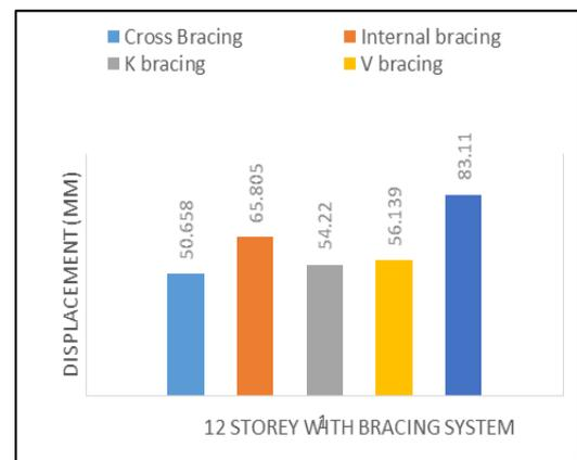
**Fig -9** Comparison of displacement for 12 storey model with bracing system.
