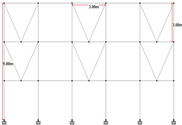
**Fig -5:** Elevation of 3 storey with V bracing.
