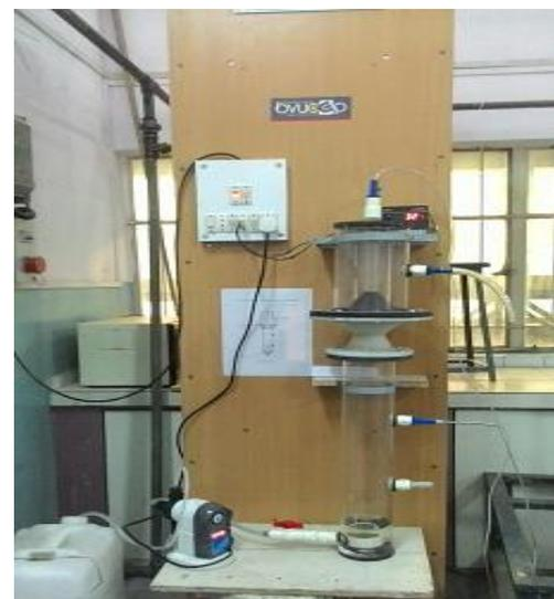
**Fig. 1** Modified UASB reactor
