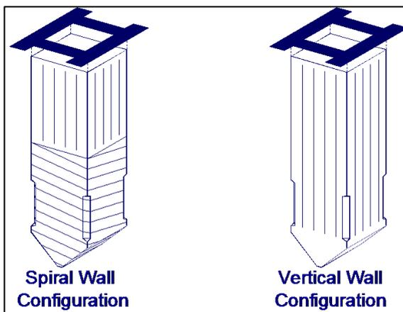
Fig. 3 Spiral and Vertical Furnace Water wall
