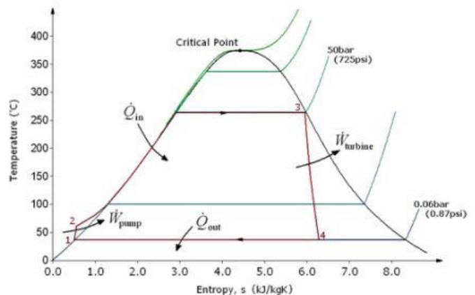
Fig 1.1. Basic Rankine cycle (with various pressures)
