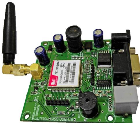
Fig -2.5: SIM800 GSM MODEM [2]
