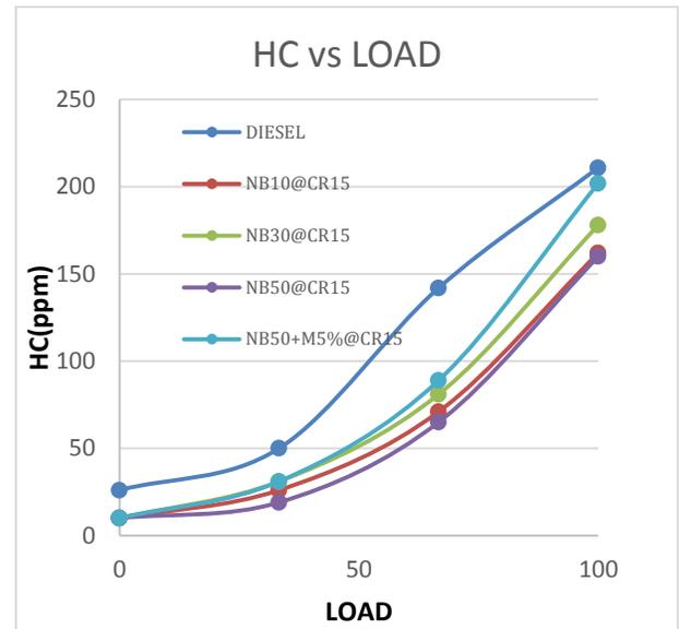
It is observed that for all the fuels tested, the HC emission is found to increase with increase in load. The incomplete combustion of the fuel due to the higher viscosity offered by the biodiesel content and poor mixing of fuel with air could be the reason for increased HC emission. From the graph biodiesels emits less hydro carbon emissions than diesel. NB50+M5% at compression ratio 15 exhibits very high HC emissions than B10, B30 and B50.
