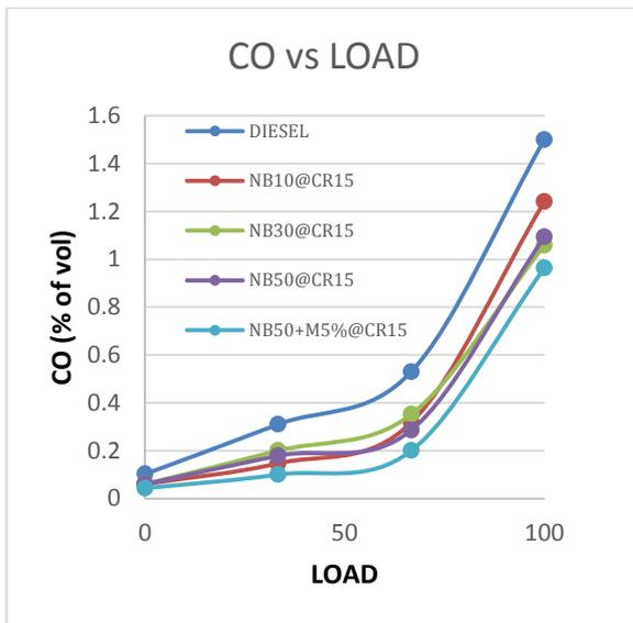
The CO emitted by all the blends is lower than that of diesel at all loads. This is due to the better combustion of the blends provided by the additional oxygen content the incomplete combustion of the fuel due to very short time available for combustion.
