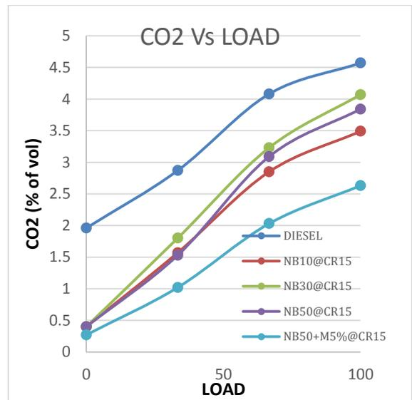
From the above graph the carbon dioxide emits very low level emissions than diesel. This is due to the fact that the biodiesel in general is a low carbon fuel and has lower elemental carbon to hydrogen ratio than diesel.
