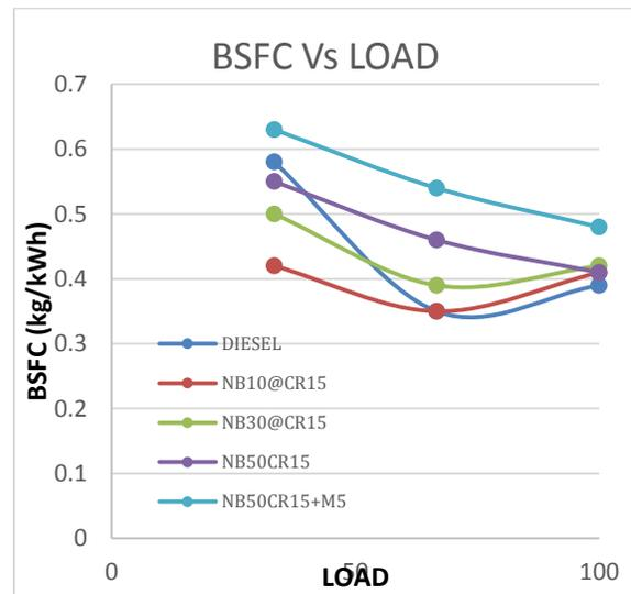
The variation in BSFC of the test fuels with respect to load is shown in figure. It is observed that the BSFC for all the test fuels are higher than that of the diesel at all loads. The BSFC for the blends NB50 without methanol at CR15 is closely to diesel. While the NB50+Methanol consumption of fuel is slightly more due to its lowest heating value.
