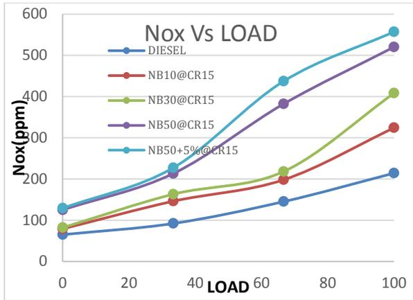
From the figure, it is observed that all the blends tested produced higher NO<sub>x</sub> emission than diesel at all loads. Also, the percentage increase in NO<sub>x</sub> emission is more at high loads.
