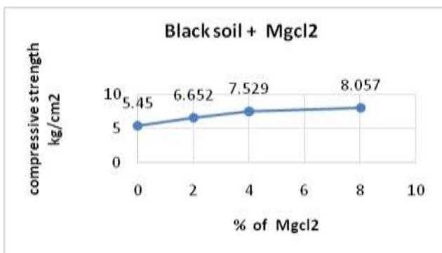
Figure 16: Variation of compressive strength with addition of Mgcl<sub>2</sub> at 0%, 2%, 4% and 8%
