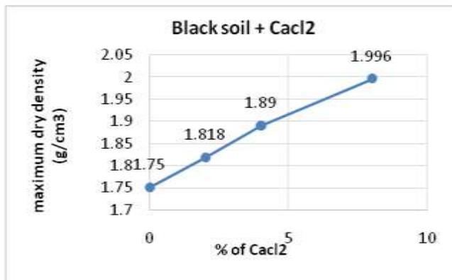
Figure 7: Variation of Maximum dry density with addition of CaCl<sub>2</sub> at 0%, 2%, 4% and 8%
