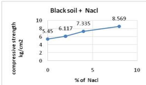
Figure 14: Variation of compressive strength with addition of Nacl at 0% ,2% ,4% and 8%
