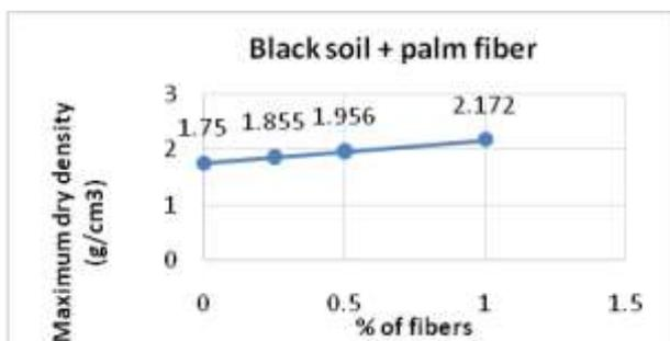
Figure 9: Variation of Maximum dry density with addition of Palm fiber at 0%, 0.25%, 0.5% and 1%
