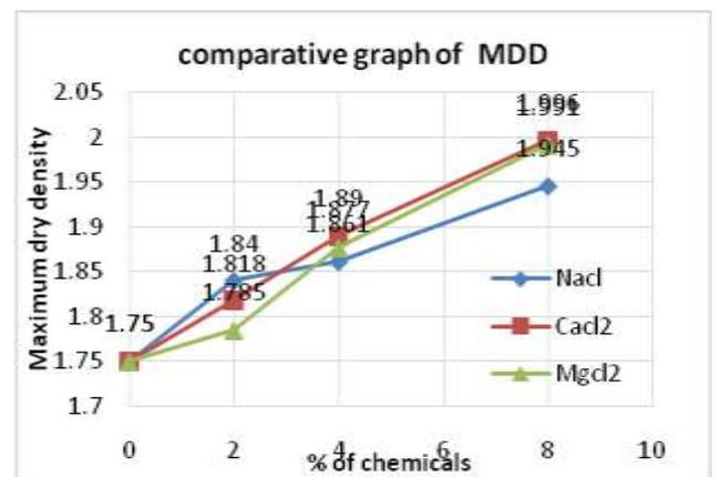
Figure 18: Combined Result of maximum Dry Density with
