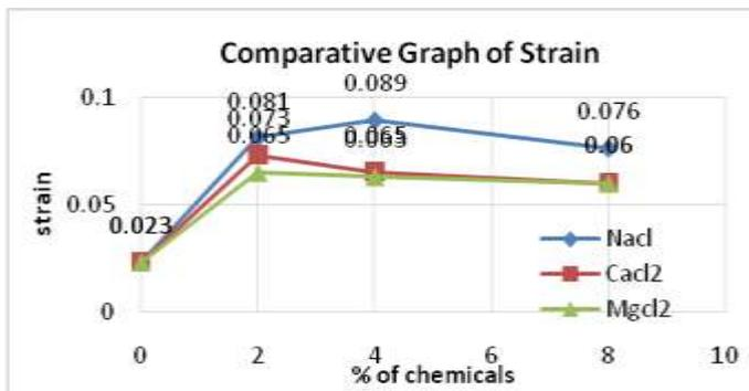
Figure 22: Combined Result of strain with all additives at 0%, 2%, 4% and 8%
