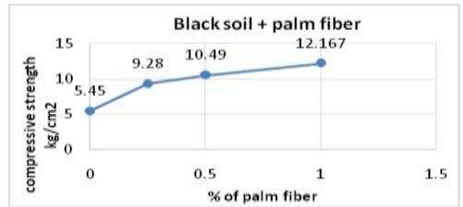
Figure 17: Variation of compressive strength with addition of palm fiber at 0%, 0.25%, 0.5% and 1%.
