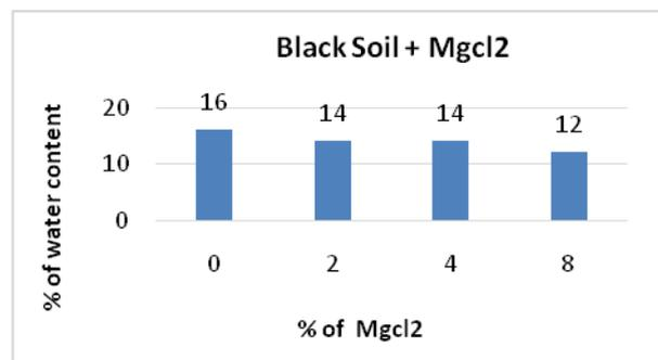
Figure 12: Variation of OMC with addition of MgCl<sub>2</sub> at 0%, 2%, 4% and 8%
