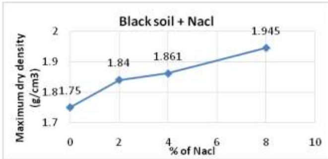
Figure 6: Variation of Maximum dry density with addition of NaCl at 0%, 2%, 4% and 8%
