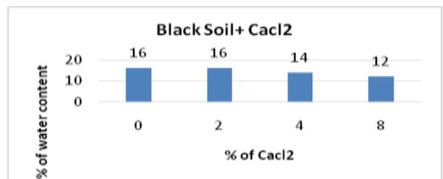
Figure 11: Variation of OMC with addition of CaCl<sub>2</sub> at 0%, 2%, 4% and 8%
