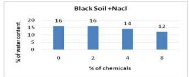
Figure 10: Variation of OMC with addition of NaCl at 0%, 2%, 4% and 8%
