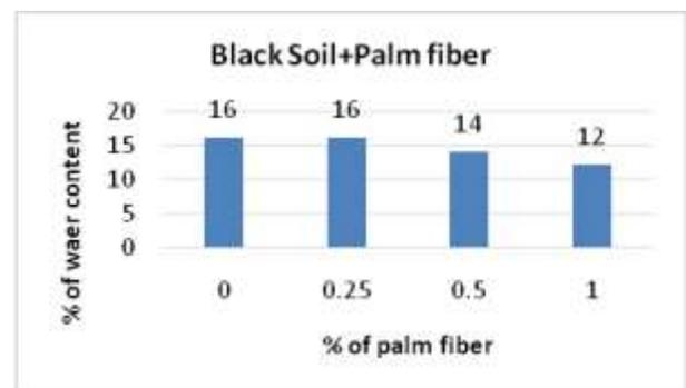
Figure 13: Variation of OMC with addition of palm fiber at 0%, 0.25%, 0.5% and 1%
