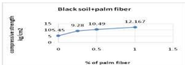
Figure 21: Result of compressive strength with palm fiber at 0%, 0.25%, 0.5% and 1%
