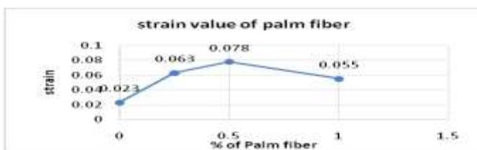
Figure 23: Result of strain with palm fiber at 0%, 0.25%, 0.5% and 1%
