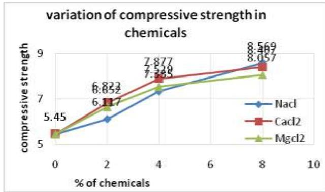
Figure 20: Combined Result of compressive strength with all additives at 0%,2%,4% and 8%
