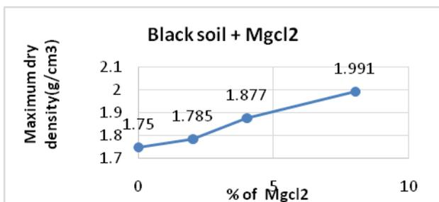
Figure 8: Variation of Maximum dry density with addition of MgCl<sub>2</sub> at 0%, 2%, 4% and 8%
