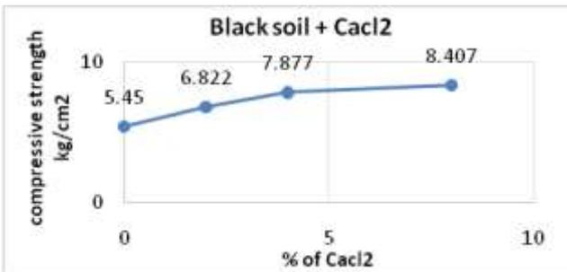
Figure 15: Variation of compressive strength with addition of Cacl<sub>2</sub> at 0%, 2%, 4% and 8%
