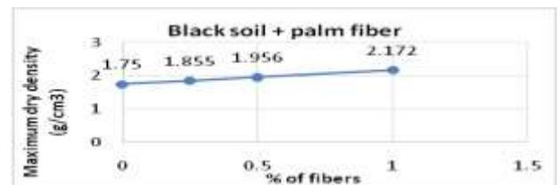
Figure 19: Result of maximum Dry Density with palm fiber at 0%, 2%, 4% and 8%
