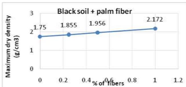
Figure 25: Maximum dry density of palm fiber
