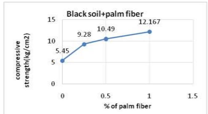
Figure 27: Compressive strength of palm fiber
