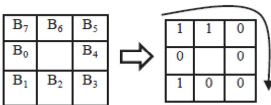
Fig. 2. input block coded in LBP
