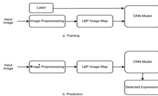
In this model, we first process the LBP image to generate the LBP feature map of the image, and then use the LBP feature map of the image as CNN input to train the CNN. Similarly, in the test identification images, it is first LBP feature map is extracted and then LBP image is fed into the CNN classifier for identification
