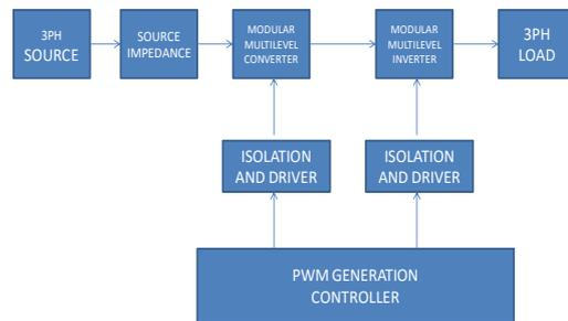
**Fig-7: MMC Modified circuit**
