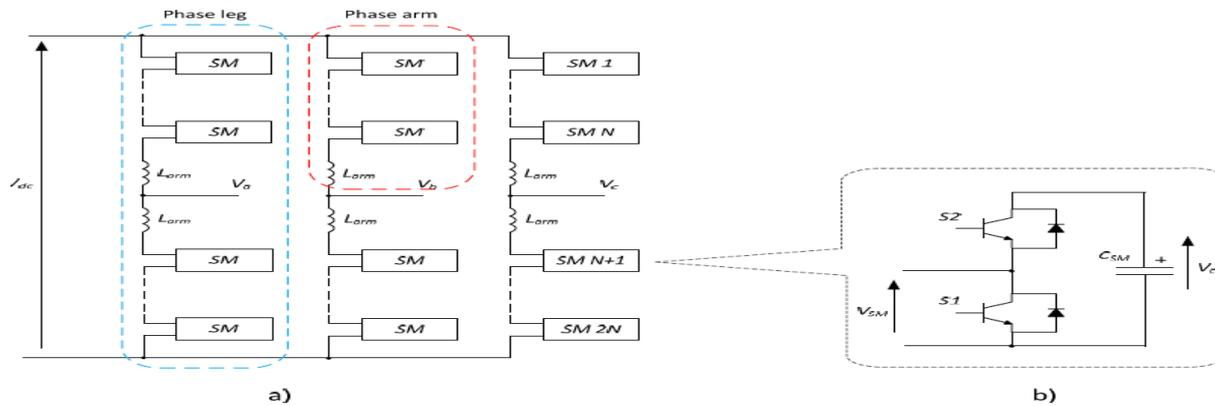
Fig-1 (a) Topology of three-phase MMC (b) Half-bridge sub-module
