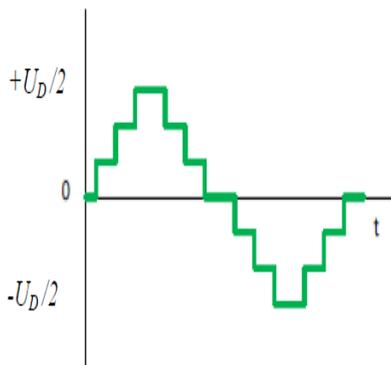
**Fig-6: Voltage waveform of a Multi-Level Converter**
