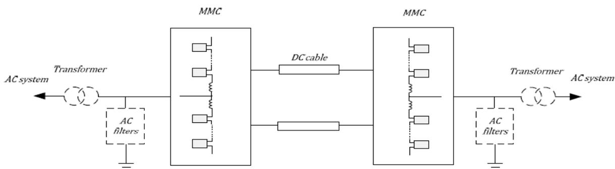
**Fig-4: MMC-HVDC system configuration**
