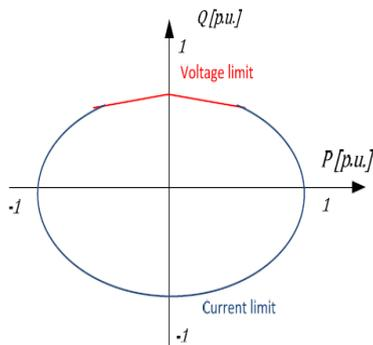
**Fig -2: Active-reactive locus diagram of VSC-HVDC transmission system**
