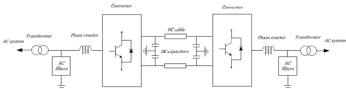
**Fig-3 VSC-HVDC system configuration**
