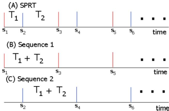
Figure 1: Staggered PRT Transmission
