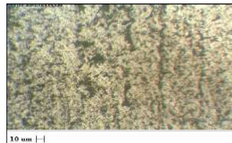
Fig-4.3 Microstructure of specimen at 1120rpm, 45mm/min.
