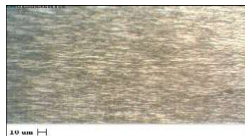
Fig-4.4 Microstructure of specimen at 1400rpm, 60mm/min.
