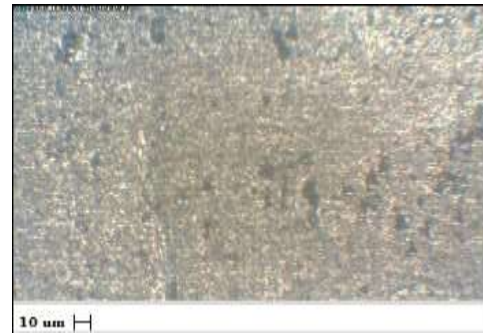
Fig-4.2 Microstructure of specimen at 900rpm, 40mm/min.
