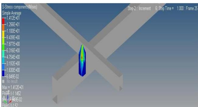
**Fig-6:** Stress analysis of existing bracket
