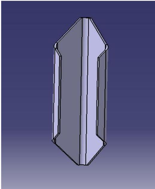
**Fig-2:** Side channel weld bracket
