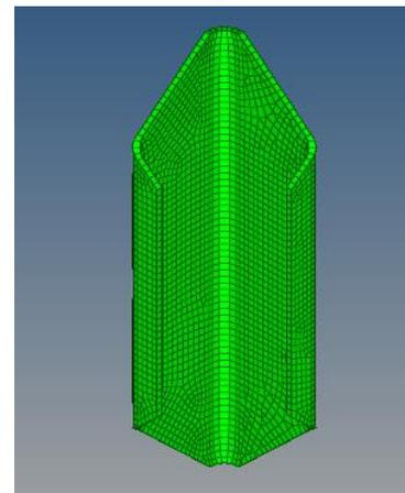
Fig-4: Meshing of existing bracket
