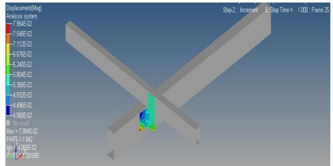
**Fig-12: Displacement of modified bracket**
