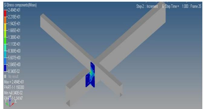
**Fig-13: Stress analysis of modified bracket**
