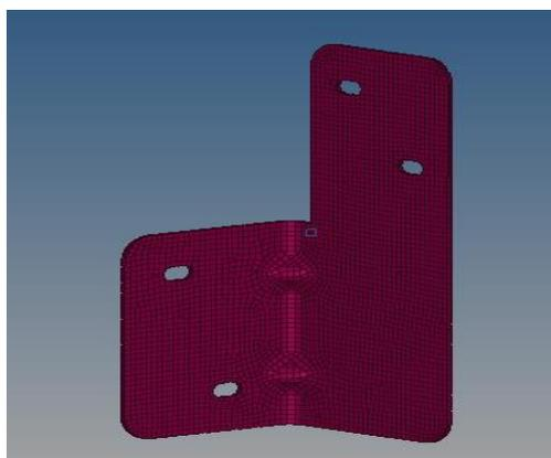
**Fig-11: Meshing of modified bracket**
