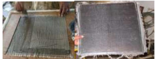
Fig -1: Preparation of specimen using hand lay up
