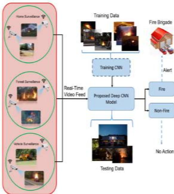
Fig. 2.1.15 Flame Detection in Surveillance videos using Deep CNN [8]
