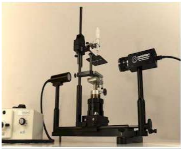
Fig. 3.1 "Ramé-hart," - 500 Advanced Goniometer Set Up
