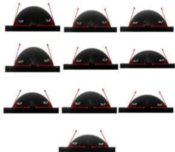
FIG. 5.1 Hydrophilic nature of CuS thin film as a function of time
