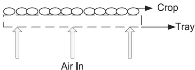
Fig-1: Thin layer solar drying
