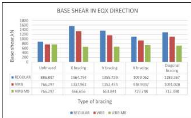
Fig no 7 – Base Shear in EQX direction
