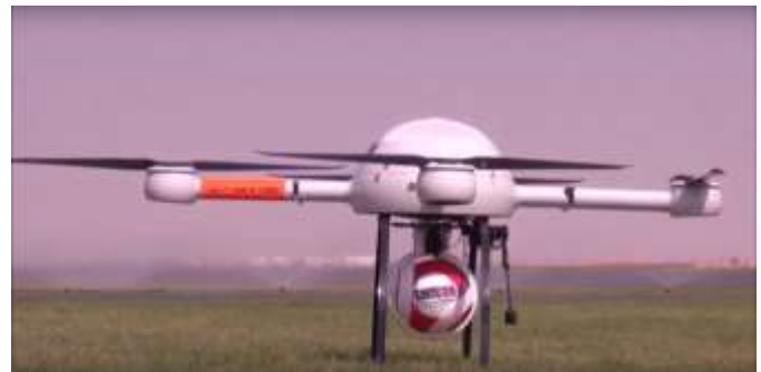
Fig 6. Fire fighter drone holding fire extinguisher ball.
