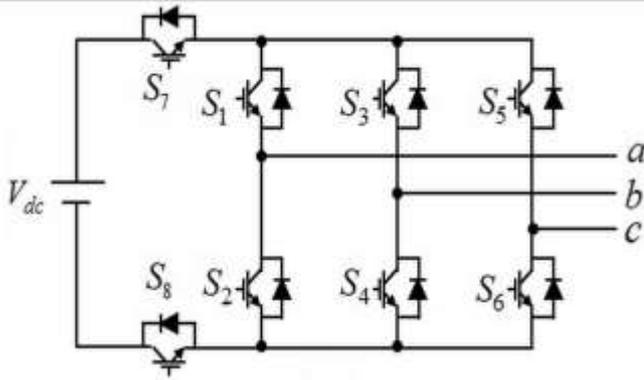
Fig-2b. Circuit diagram of the H8 inverter
