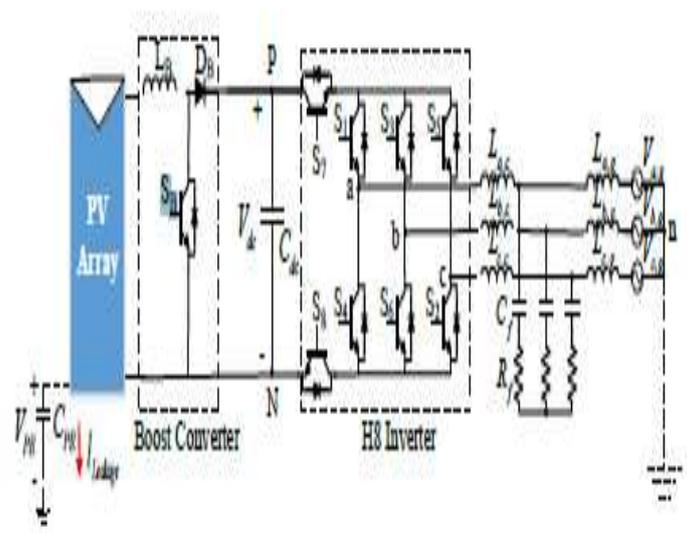
Fig-2a. Circuit diagram of the proposed system
