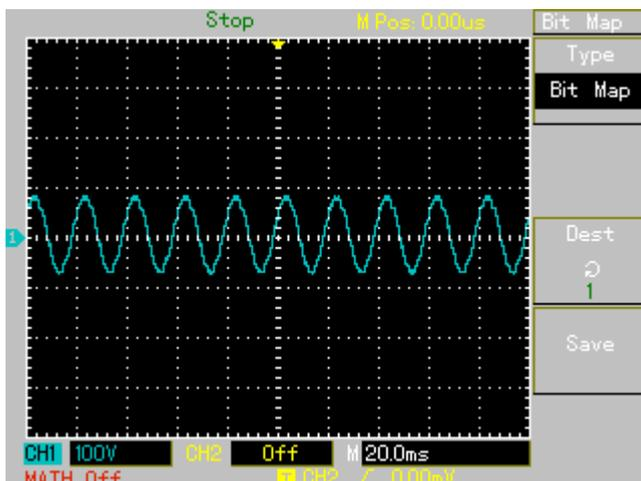
Chart-4 One Phase Output Voltage of H8 inverter using DSO
