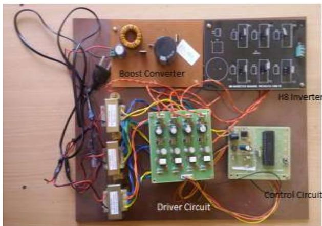
Fig-4 Hardware Section
