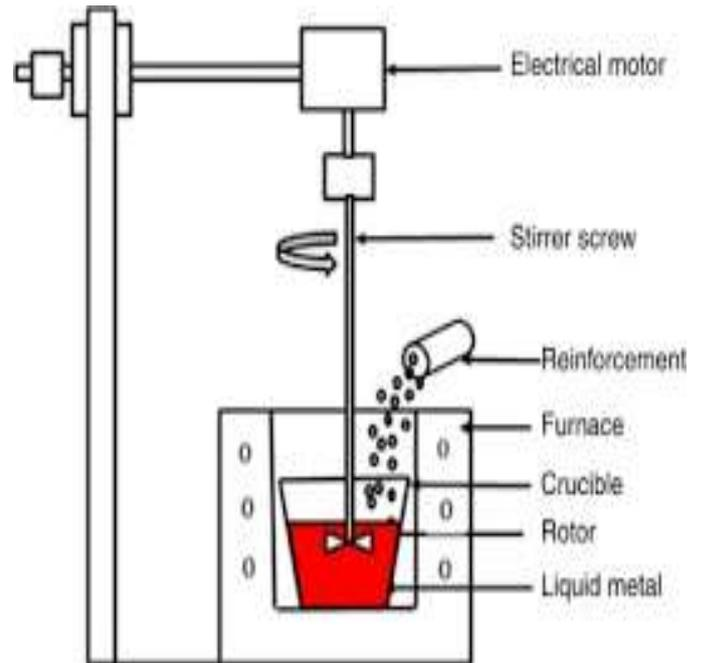
**Fig-4: Stir casting**
