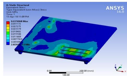
Fig -13: Stress in Base plate
