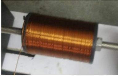
**Fig- 15** : Armature after winding
