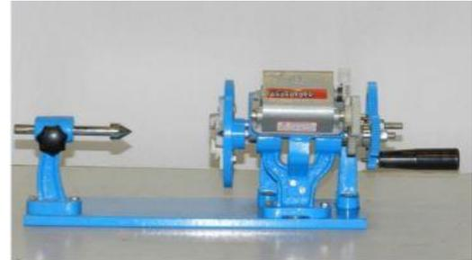
Fig - 1: Manual Coil Winding Machine
