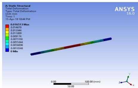
Fig -10: Deformation of Threaded Shaft
