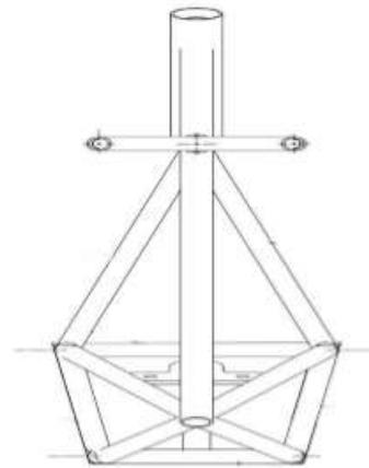
Fig -2: Front View Design of Steering Mechanism
