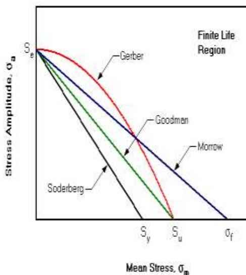
Figure 6: Comparison of Mean Stress Equations.
