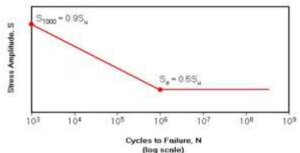
Figure 3: Generalized S-N Curve for Wrought Steels.
