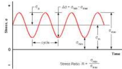
Figure 4: Typical Cyclic Loading Parameters..
