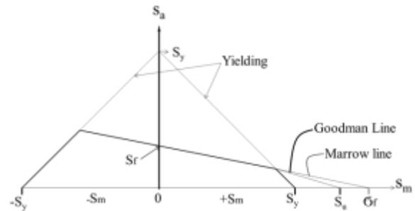
Figure 7: Fatigue and yielding criteria for constant life of unnotched parts.
