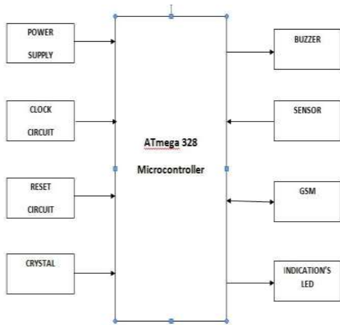
Fig -3: Functional Block diagram
