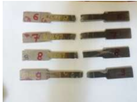
Fig-7: Samples after tensile test
