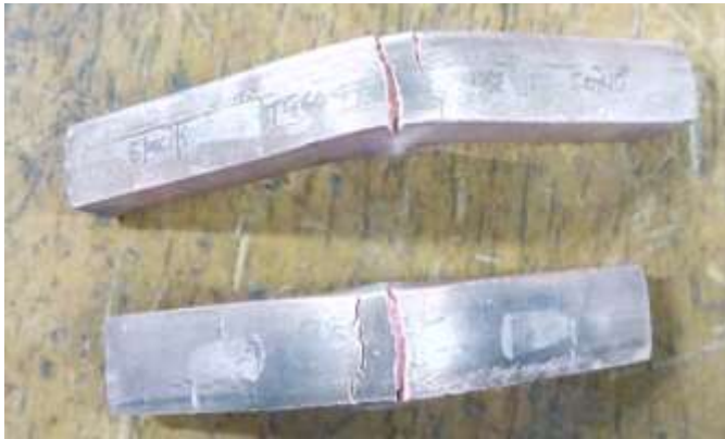
Fig .3 Samples failed in Close bend test after heating in hydrogen atmosphere at a temperature of 850 deg C for 30 minutes (ASTM B 577 Method C). Cracking during bend test shows the presence of hydrogen embrittlement
