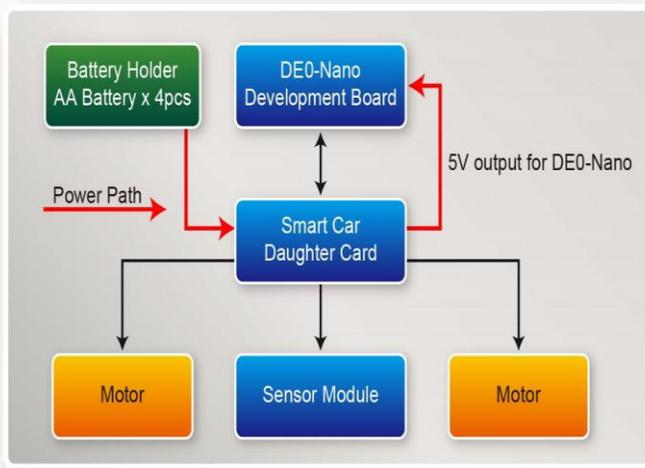
A line follower Car is mainly a combination of three boards, the chassis, motor and other components combined. Below we will introduce the three boards. The first board to be introduced is the main controller called Terasic DE0-Nano Board. This board uses the Altera
