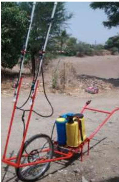
Fig -7: Vertical Lance Arrangement
