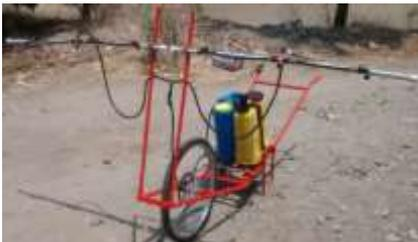
Fig -6: Spraying Pesticides by Horizontal Lance
