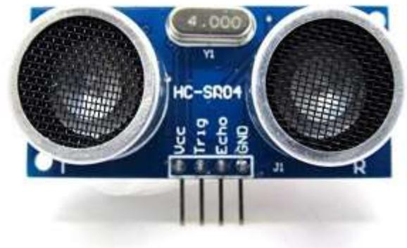
Fig -4: HC-SR 04 Ultrasonic Distance Sensor.
