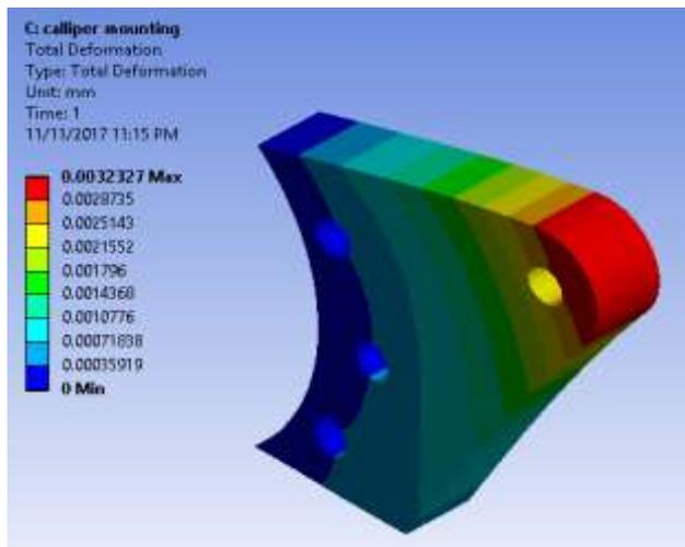
**Fig -9** Caliper Mounting deformation analysis
