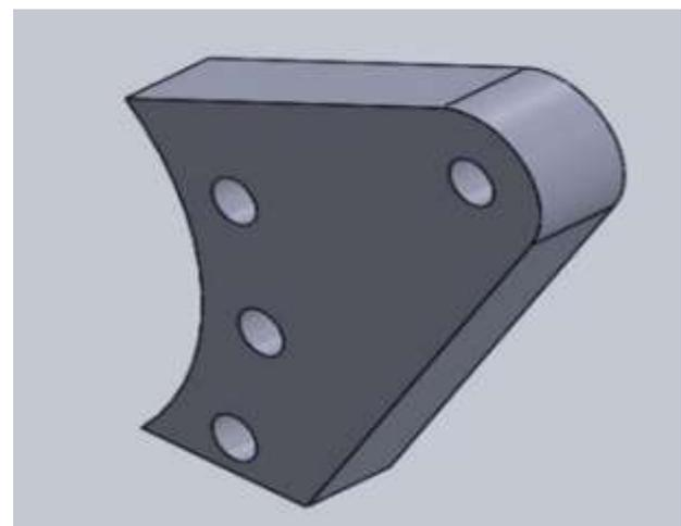
Fig -7: Caliper Mounting
