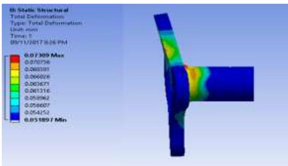
Fig -3: Wheel Hub Deformation analysis
