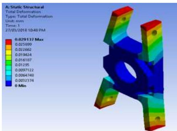
Fig -6: Rear upright Deformation analysis
