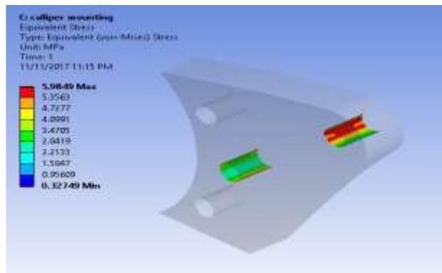
**Fig -8:** Caliper Mounting stress analysis
