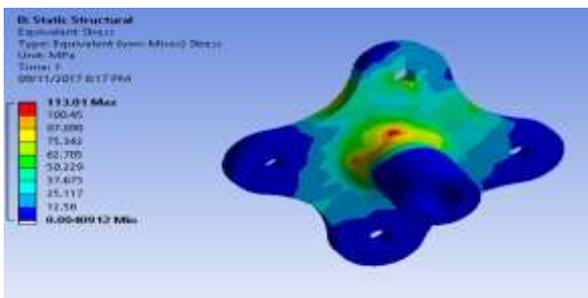
Fig -2: Wheel Hub stress analysis
