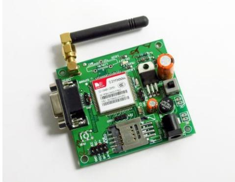
Figure 1: GSM module
