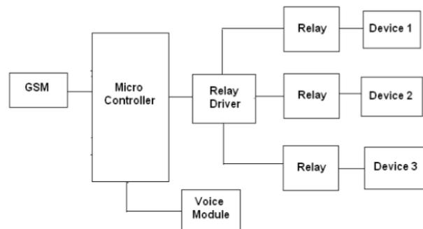
Figure 3: Block diagram of GSM based IVRS system
